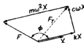
FIGURE 3.6.1. Disturbing force transmitted through springs and damper.
